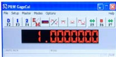
The operator simply chooses the class of gage (ie., XX or XXX), in the dialogue box, selects the appropriate cell in the "smart" spreadsheet, and clicks on the *close probe* icon (or presses the footswitch). GageCal™ displays the measurement in the "Current Reading" window and automatically updates the record. The data can be saved, printed in a customized report, or exported to many popular gage management software packages.
